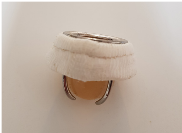
Fig. 3 Photograph shows a Pemco-Cartwright valve, with an incomplete 4-strut cage and a Silastic ball.
