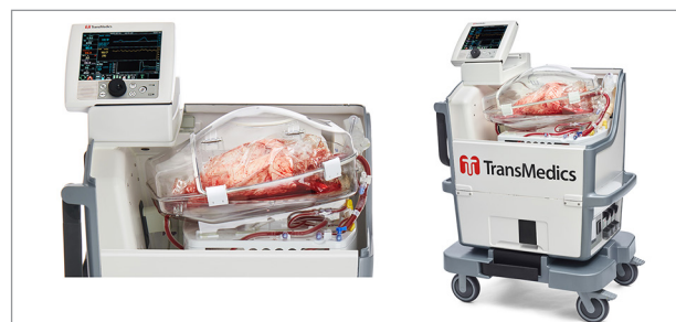
Fig. 1 The TransMedics Organ Care System (OCS), a portable ex vivo lung perfusion system, enables ventilation and perfusion of the donor lung throughout transportation. (Photo courtesy of TransMedics, Inc.)
